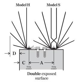
Use Model H with Model S on the following surface sizes: Single exposed: 4" to 6-1/2" deep - Double exposed: 3-1/2" to 6" deep
