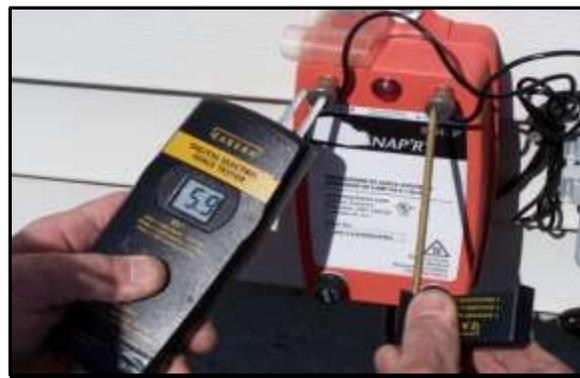
Reading voltage with the entire ShockTape system connected.
