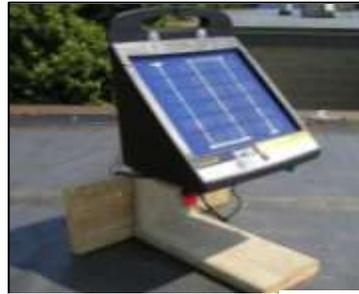
Stand made from a 6 foot long x 5/4" x 6" deck board.
