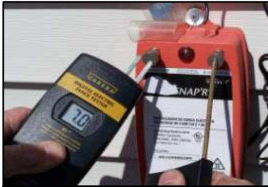
Reading voltage of the line charger while disconnected from the system.
