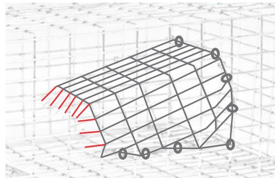
Bend the wires inward to narrow opening at the small end so birds can't get back out the door
