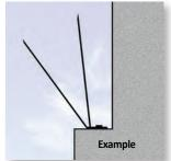
Installs on narrow surfaces with optional hardware or glue clips and adhesive.
