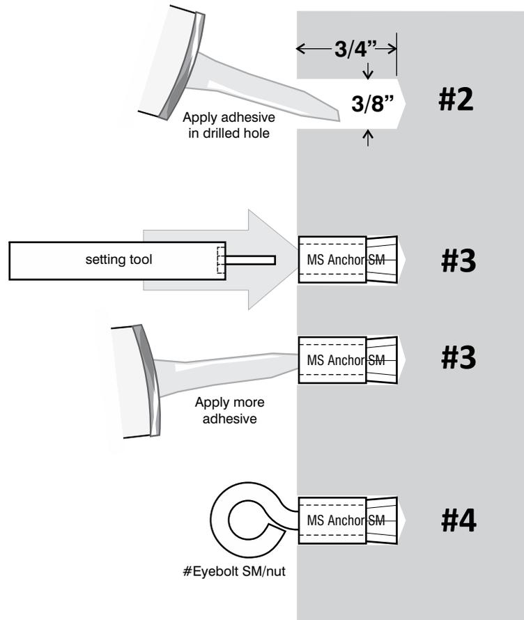
**#1.** Mark the location of each cable guide (2' center-to-center or less). To secure the Small Eyebolt (#Eyebolt SM/nut), you will need to install the small Machine Screw Anchor (#MS-Anchor SM). Both eyebolt and anchor have 10-24 threads.
