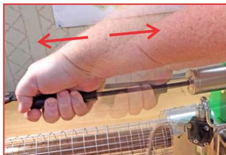
While pressing the Starter Button, cycle Air Pump until the fogger starts. Keep pumping for 10 sec. after it starts.
