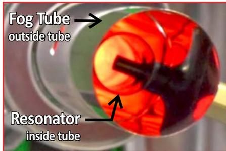
**When properly tuned, the exhaust flame does not go past the end of the Resonator tube (smaller inner tube).**
