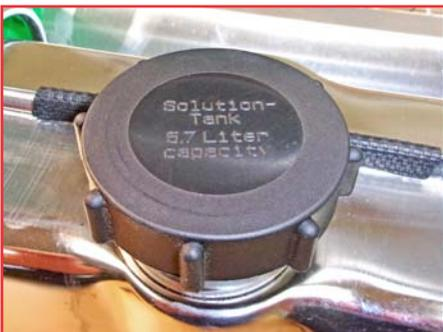
Slowly open the Solution Tank cap to depressurize the tank. You should hear a hissing sound.
