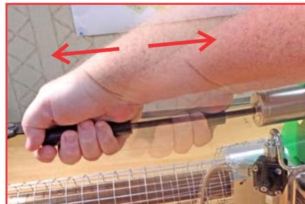
With the Fuel Button OFF, hold the Starter Button ON and pump the Air Pump until the fogger stops popping.
