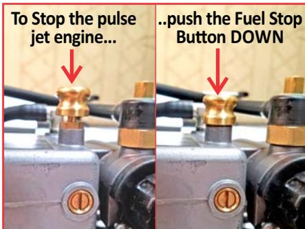
To stop the fogger, push the Fuel Stop Button DOWN which stops the gas to the engine.
