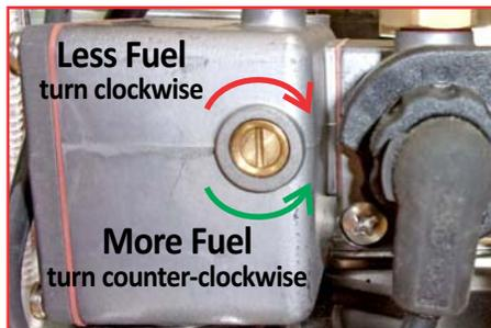
**Adjust the exhaust flame by turning the Regulating Needle screw. The flame should be just inside the Resonator.**
