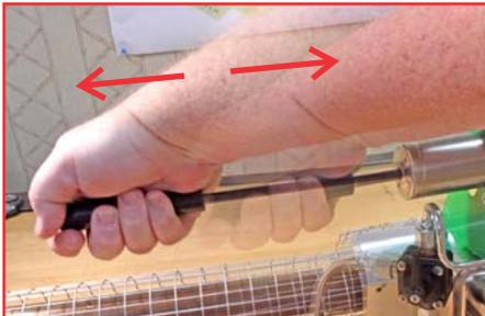
Before starting the fogger, press the Starter Button and cycle the Air Pump a few times to build pressure in the tanks.
