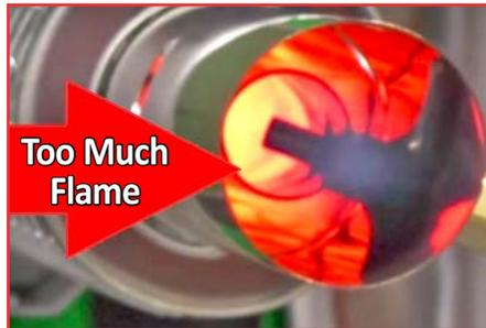
**If the flame goes past the end of the Resonator you must reduce the amount of fuel with the Regulating Needle.**
