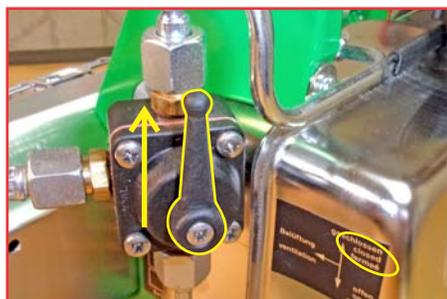
**The Solution Tap Valve is at the front of the Solution Tank. When the valve handle points UP, the Solution Tap Valve is CLOSED.**
