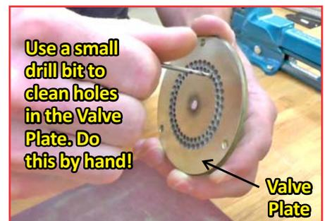
If the holes in the Valve Plate are dirty or clogged, clean them BY HAND with a small drill bit.
