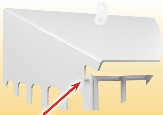
The drop-notch front gate (patent pending) makes access for brushes and duct cleaning equipment a breeze. With the easy opening vertical bar gate, there's no need to remove fasteners from the wall for cleaning.
