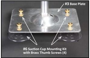
To mount the reflector on a no-drill surface (like the roof of a car or on a glass surface) you can purchase the Suction Cup Mounting Hardware Kit (#6) to hold the reflector in place. To install, pass the brass thumb screws through the four mounting holes in the Base Plate (#3), then screw on the suction cups.
