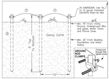
Diagram 1 - Ground System Installation
