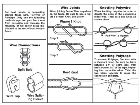
Diagram 6 – Wire Splicing and Connections
