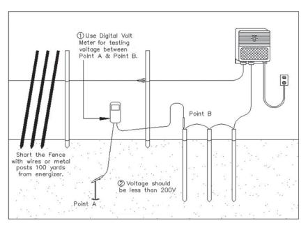
Diagram 3 – Testing the Ground System
