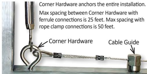
Corner Hardware anchors the entire installation. Max spacing between Corner Hardware with ferrule connections is 25 feet. Max spacing with rope clamp connections is 50 feet.
