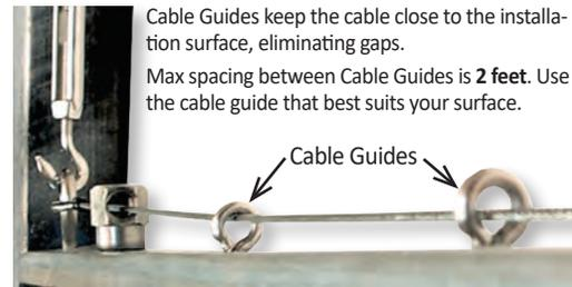
Cable Guides keep the cable close to the installation surface, eliminating gaps. Max spacing between Cable Guides is 2 feet. Use the cable guide that best suits your surface.
