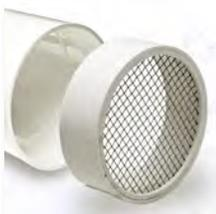
Stop wildlife, leaves and debris from getting in PVC vent pipes. Available in 2", 3", 4" and 6" sizes. Made from Schedule 40 PVC with a 3/16" stainless steel mesh screen. Attaches to schedule 40 PVC fitting or flange (not included).
